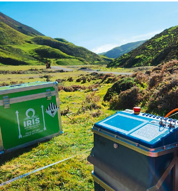
The Syscal Terra next-generation resistivity meter, used by RDCL in New Zealand. © ALISTAIR STRONACH
